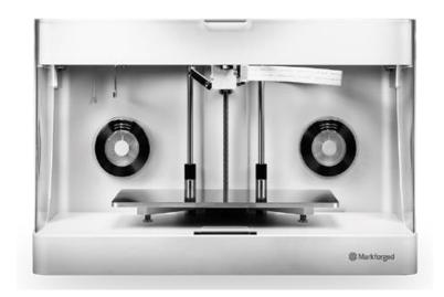
The Mark Two uses a patented Continuous Filament Fabrication (CFF) process to reinforce 3D printed nylon parts with automatically contoured and optimized toolpaths of continuous strand carbon fiber, Kevlar, and fiberglass. Utilizing a dual head system with a CFF print head and an FFF (Fused Filament Fabrication) extrusion head, the Mark Two can create astonishingly robust parts by leveraging the properties of composite materials with a higher strengthto-weight ratio than 6061-T6 Aluminum.
